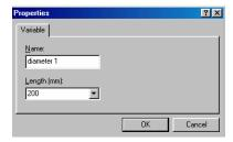
Change the Length value to a diameter of 200 mm and click on OK to complete the command.
