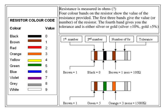
Work out the resistance (in Ohms ?) of the following resistors. Disregard the tolerance band (gold or silver band)
